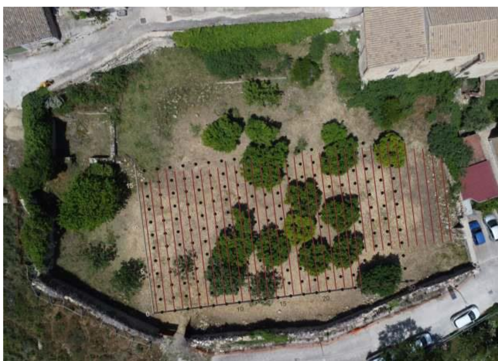
Fig. 3. Aerial view of the “Giardino dell’Annunziata, in Cammarata. The black dots indicate the ERT electrode positions. The red lines indicate the GPR profiles.
